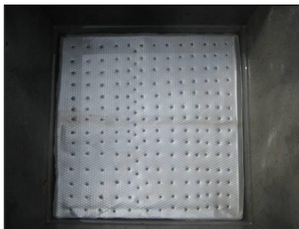
This is an example of a bad diffuser. It has too many holes - only 100 holes are needed.
